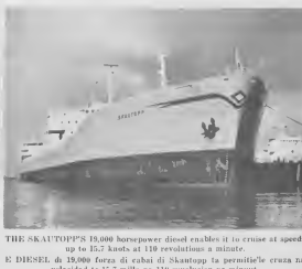
THE SKATOPP'S 18,000-horsepower diesel enables it to cruise at speeds up to 15.7 knots at 110 revolutions a minute. E DIESEL di 18,000 forsa di cabal di Skatopp ta permitie e crusa ta velocidad te 15.7 milla na 110 revolution pa minuto.
